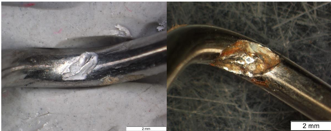
Fig. 6. Typical tribocorrosion in the friction area of a stainless steel net after some months in the Pacific Ocean
